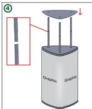
Connect the Pipe #3 and #4 on the table top and then put on the shelf, repeating this until the 4th layer.
