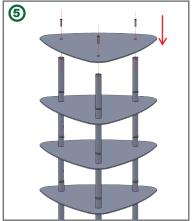
Install the screw on the Pipe #6 and the last layer
