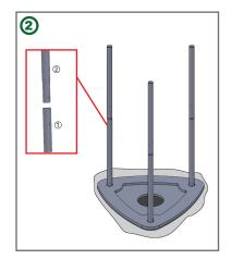
Connect the Pipe #1 and #2, inserting them into the slots in base
